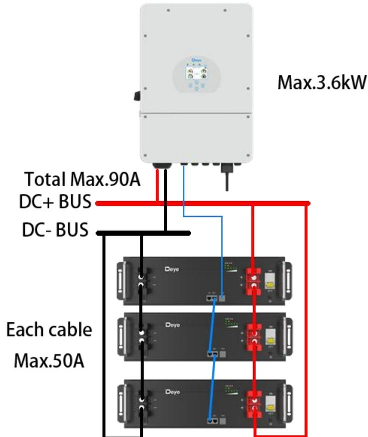
If the inverter power exceeds 3.6kW, the parallel mode must be used mode 2!
