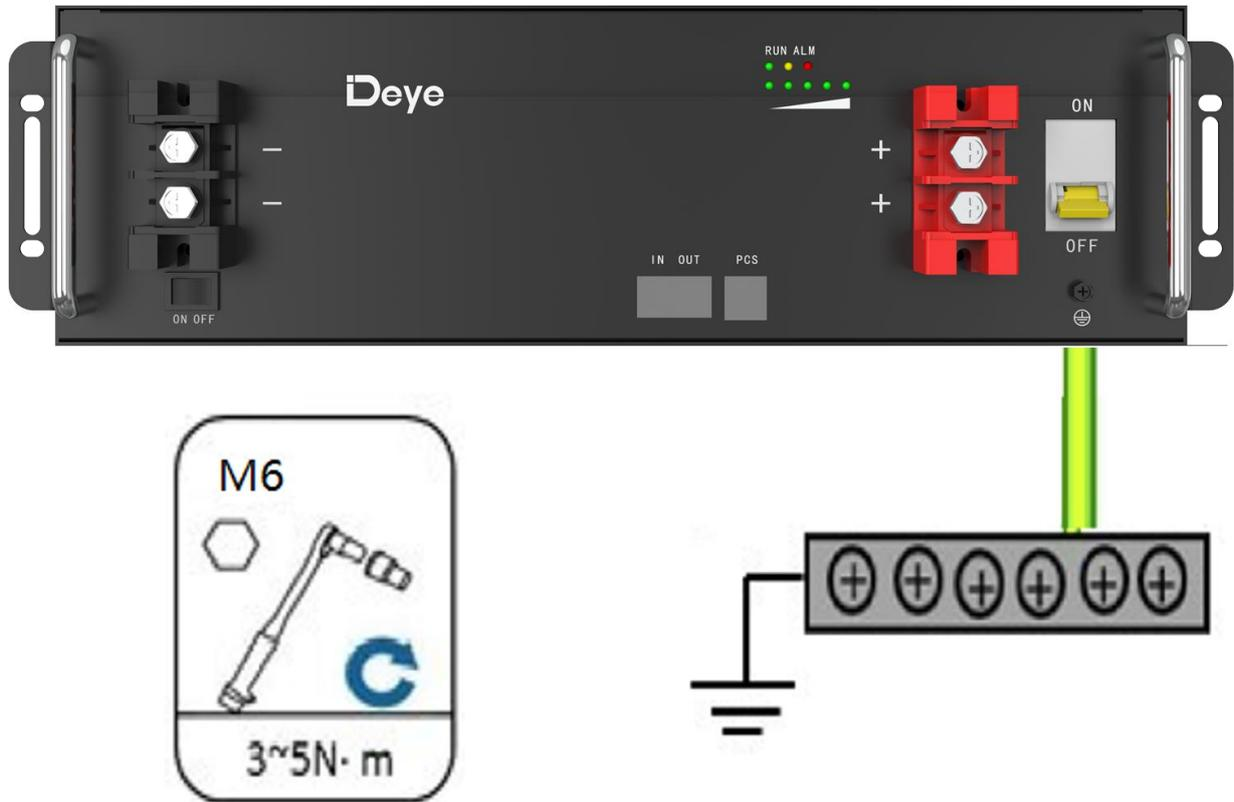
Figure 5-1: Install the Grounding Wire
