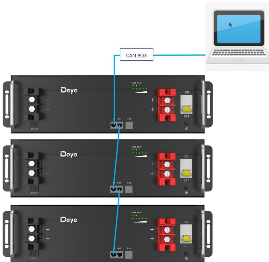
Figure 5-3: Communication Cable Connections between Battery and Computer
