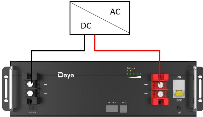
Figure 5-2: Single Battery Connection
