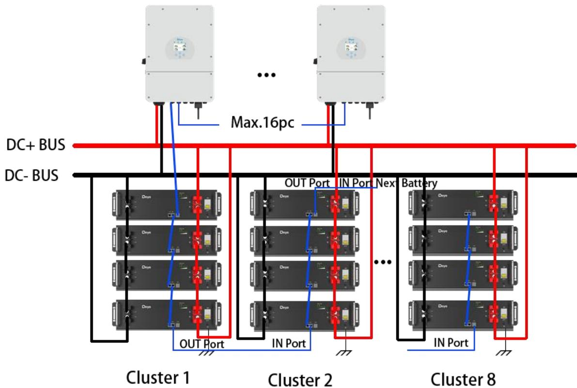
**5.2.2. As shown in 5.2.1, connect the communication line (a standard RJ45 network cable) between the adjacent batteries.**
